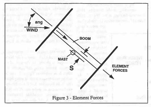
about element torque. The position of elements on the boom is not important. At first this seems counter to common sense. But when you know the element forces are down the boom centerline, it's clear that element position isn't important.
