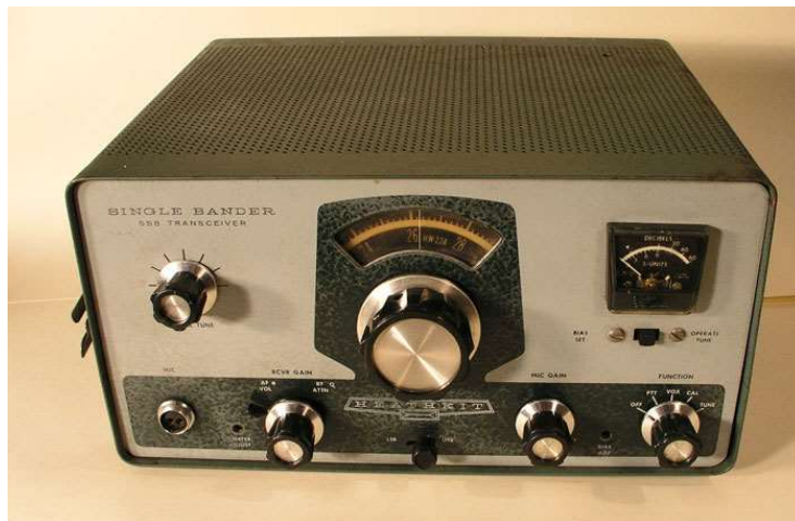
1. The Heathkit line of low-cost, high-frequency SSB receivers, transmitters, and transceivers used vacuum tubes. (Source: https://www.qsl.net/sp5btb/vintage.html )
