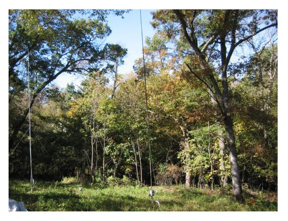
**#1:** Phased verticals aimed 30 degrees for EU, broadside to Asia. The DXE 40m is left while the 80-6m BigIR MK3 is on the right. Note the phase switch in-between the two
