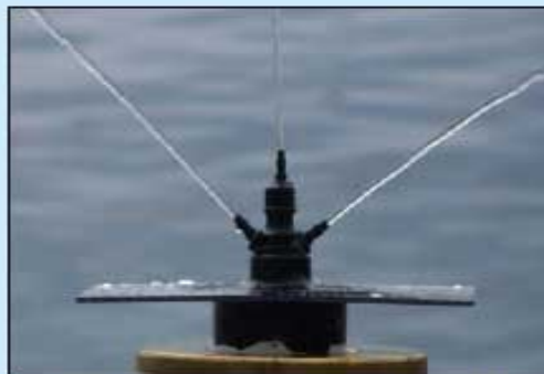
A stream of salt water can be used to transmit and receive signals over various frequencies
