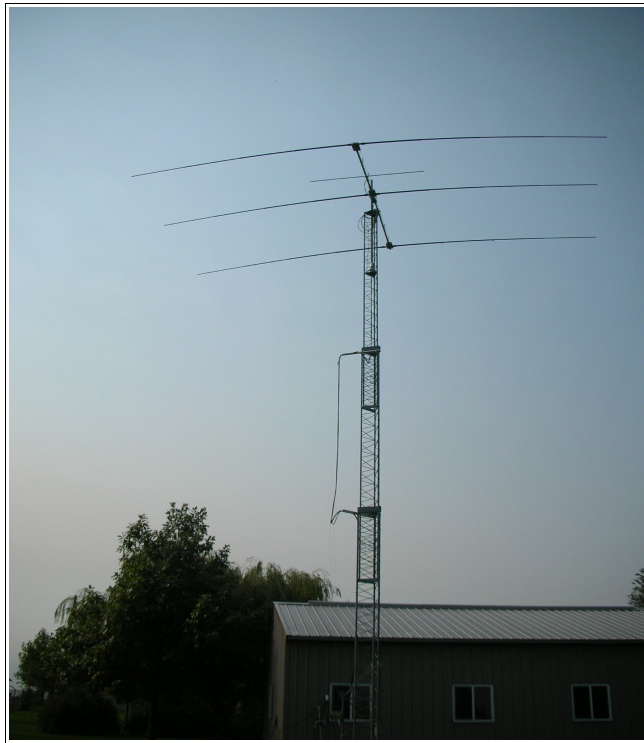
Rich Haendel, W3ACO. 3 element SteppIR with 6 meter parasitic element on a Tashjian 54 ft crank up tower.
