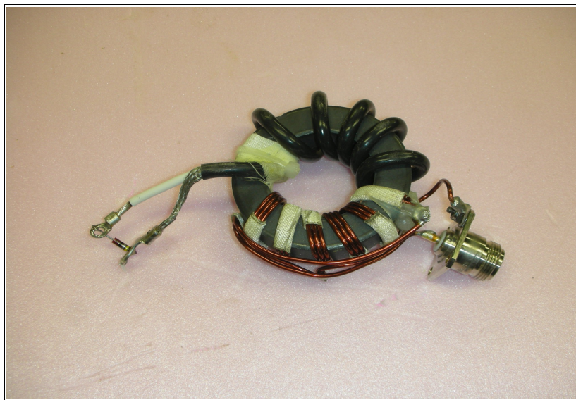
Figure 2 50:22 ohm transformer and balun with 22 ohm load
