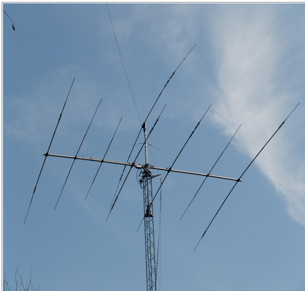
Gary Huff, KWØJ: Hi-Gain TH-7, Cushcraft D3W, and a G5RV Dipole. Also has the M/2 6 meter HO Loop at 40' and 2 meter Ringo Ranger II.
