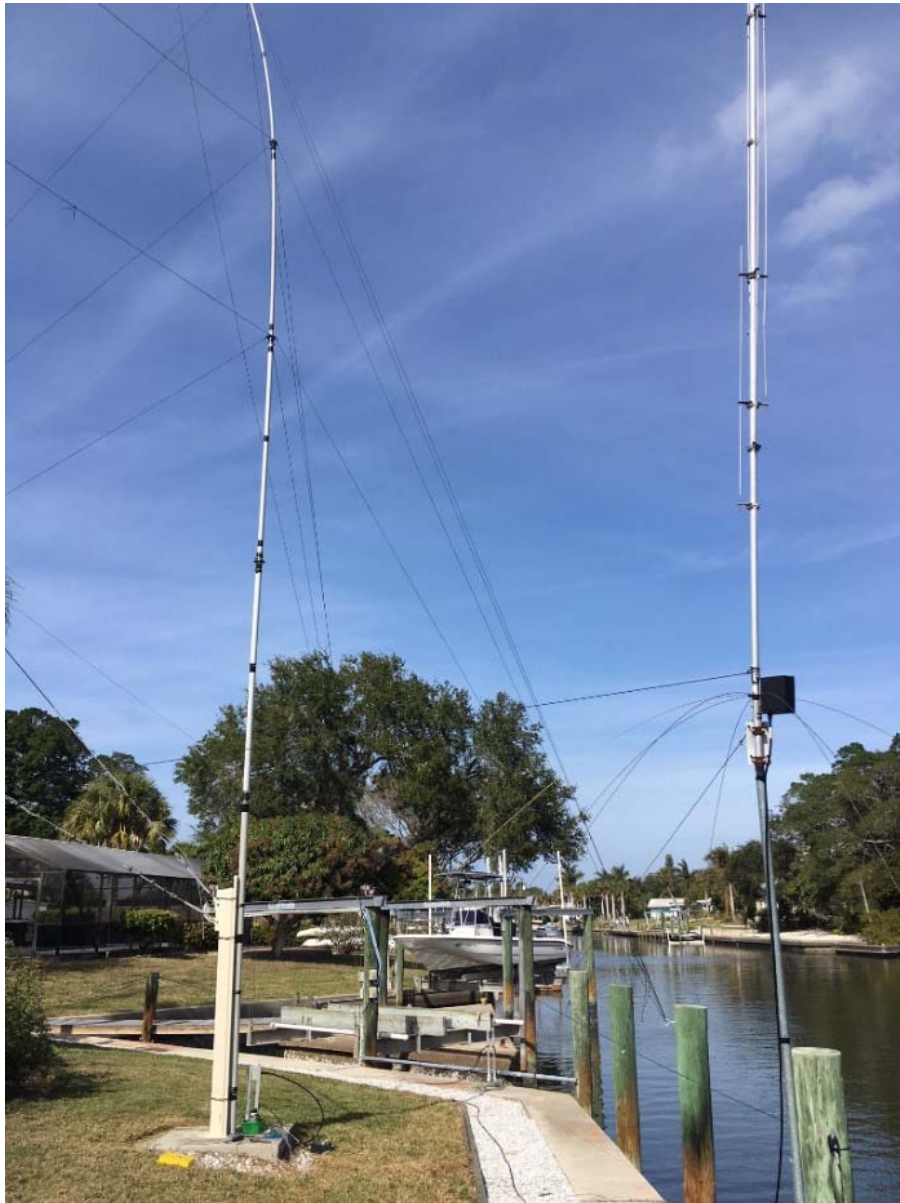
Left - part of the 160m inverted L; right - vertical mounted dock-side. All radials end in the salt water canal.
