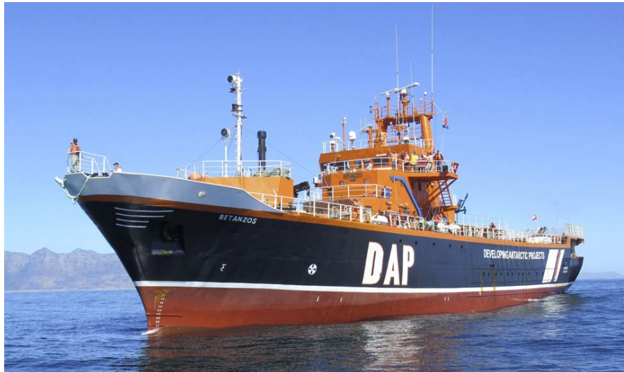
M/V Betanzos, 236 feet long, 41 feet wide, Gross tonnage 1438T, built in 1973
