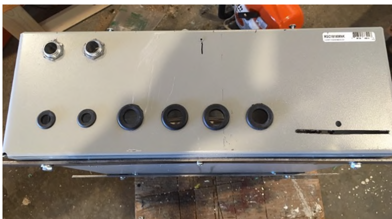
The slot on the right is for the 6" wide copper strap that will be attached to the ground system
