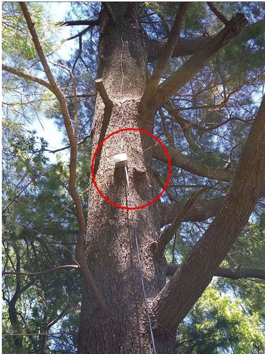
Figure 2 - Close-up of the feedpoint showing radial wires
