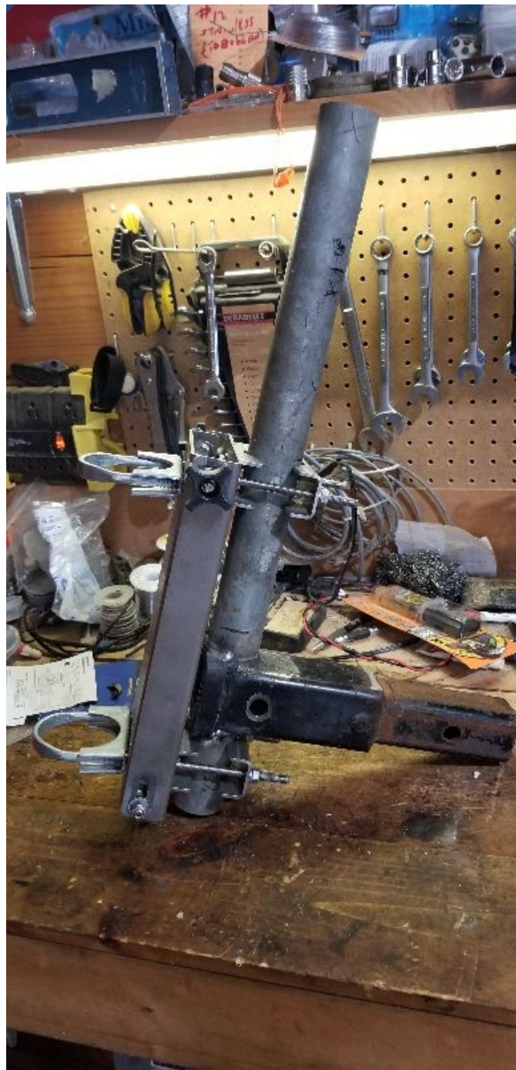
The 2" receiver extender with two pieces of 2" mast welded on the top and bottom. The DXE Omnitilt now mounted solidly to the extender with 2" clamps. The empty clamps are the 2.25" galvanized U-Bolts for the Rohn mast.
