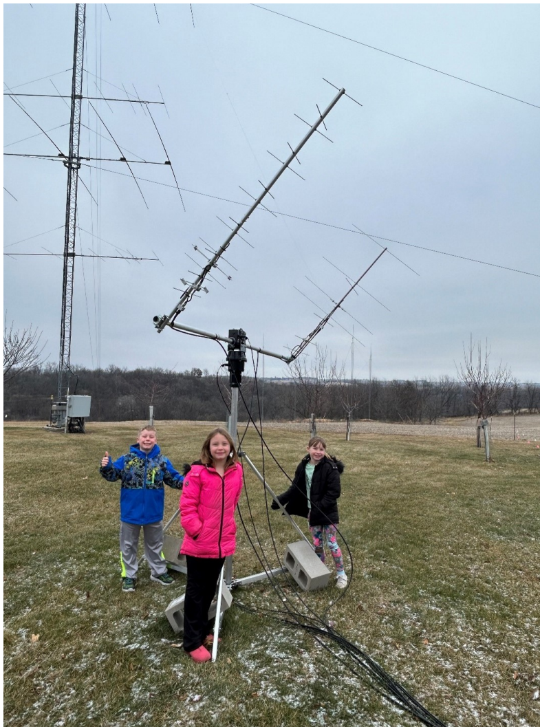
LEO pack antenna, Yaseu G5500 AZ-EL rotor on tripod. WØGJ's secondary harmonics, 7-year old triplets for size comparison. Great helpers!!!
