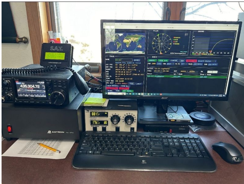
WØGJ satellite station. ICOM 9700 with S.A.T. controller (and it's display), Green Heron AZ-EL rotor controller, monitor is sitting on an old mini-computer.
